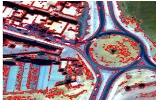
Figure 4.(c) segmented image \delta=0.2 \Phi=5 number of iterations =150
