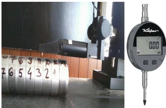
Fig. 5. The measuring device for measuring the roughness of processed surface TALYSURF-INTRA and the device of vibration measurement – Comperator
