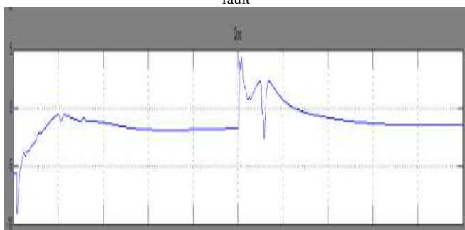
Fig. 10. MATLAB_SIMULINK output for Q_{RSC} during three phase fault
