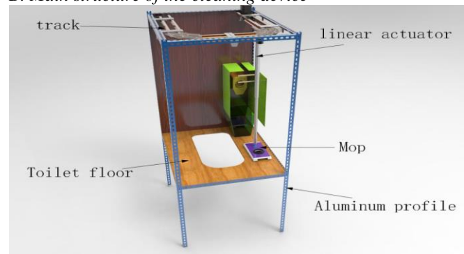
Figure 1 Model of cleaning device at working status.
