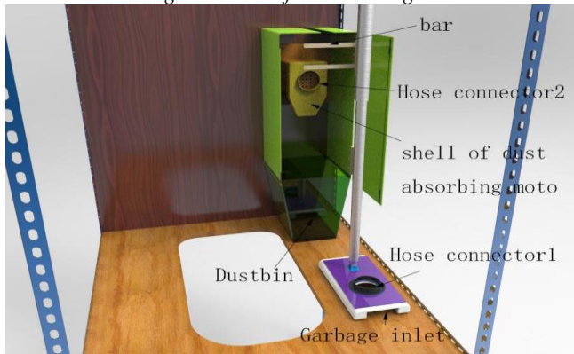
Fig. 10 Dust absorbing structure of the device.
