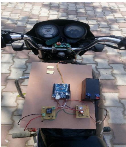
Fig. 4.1 Arrangement Diagram in Hero Splendor plus
