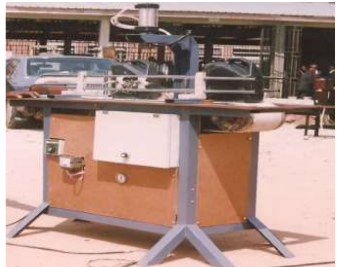
Fig 15: Photograph of sealing machine
