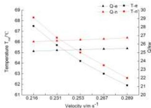
Fig 10: Heat recovery variation with fluid velocity
