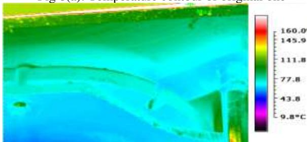
Fig 6 (b): Temperature contour of Water cooling type
