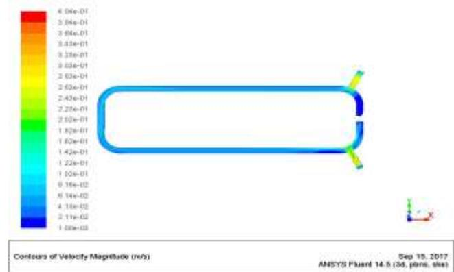
Fig 3(a): Fluid velocity contour on upper side
