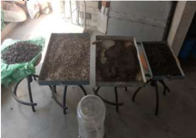
Fig. 16: Materials used in slow sand filter
