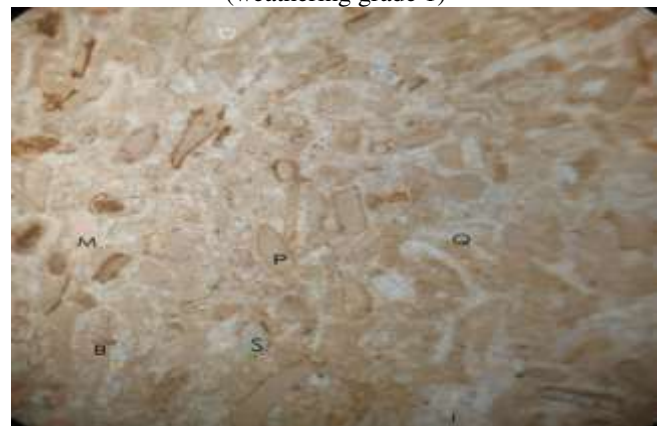
Figure 2: Photomicrograph of Limestone (weathering grade 1)
