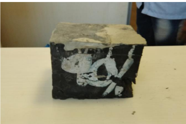
Figure 6. 90% LDPE plastic beads + 10% fly ash bricks
