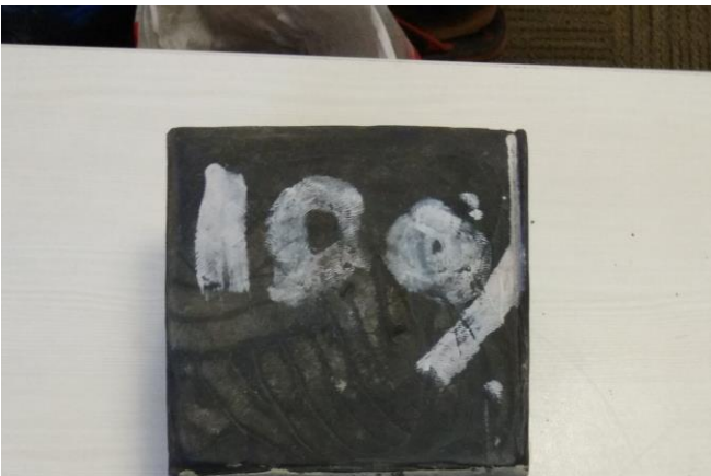
Figure 5. 100% LDPE plastic beads bricks
