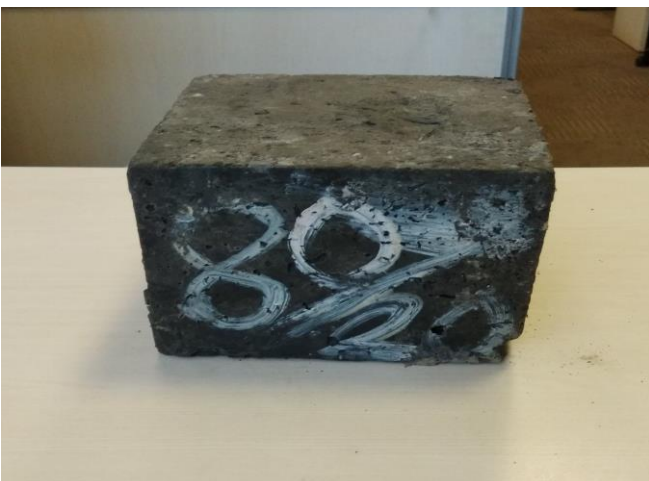
Figure 7. 80% LDPE plastic beads + 20% fly ash bricks
