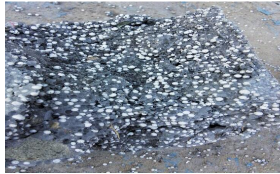
Fig.5.Failure interface of recycled aggregate concrete destruction of the interface between the cement mortar and the EPS particles, and less the interface failure between the aggregate and the fresh cement mortar. The specimen is in a state of unconfined compression so that the edge of the test piece is pulled away to form a penetrating seam, and the interface destruction morphology is as shown in Figure 5.
