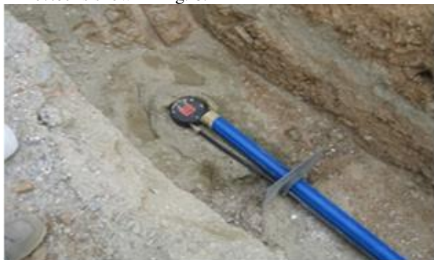
Fig. 6: Horizontal Movement Gauge
