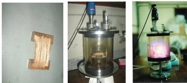
Fig. 1 Schematic diagram of jute fibre and position of it in the glow discharge reactor
