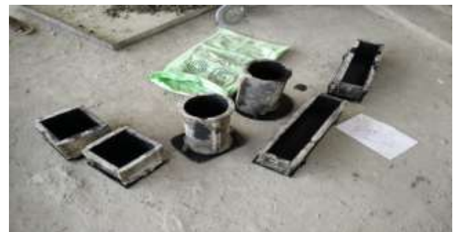
Fig 3: Samples of Cubes, Cylinders & Prisms
