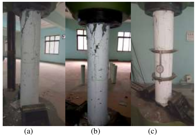
Fig 10: (a) Failure of 100% GFRP Column (b) Failure of Partial GFRP Reinforced Column (c) Failure of Conventional Steel Column
