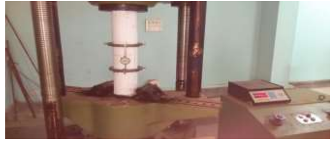
Fig 7: Showing Loading Arrangement for Short Columns under UTM
