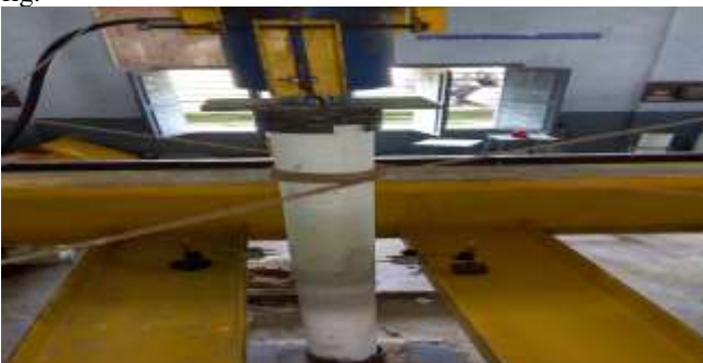
Fig 6: Showing Loading Arrangement for Columns under Loading Frame
