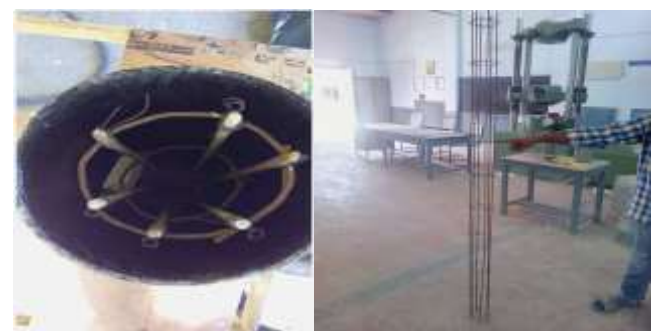
Fig 4: Showing Reinforcement Detailing and Arrangement Long and Short Columns of HYSD Steel & GFRP Rebar's In PVC Pipe
