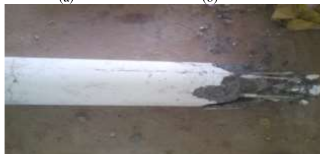
Fig 15: Failure of Long Columns in (a) GFRP + STEEL with GGBS Column (b) Conventional Steel Column (c) 100% GFRP Rebars Column
