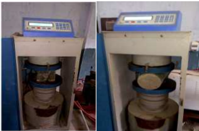
Fig 5: Showing Compression Test of Cubes under & Cylinder
