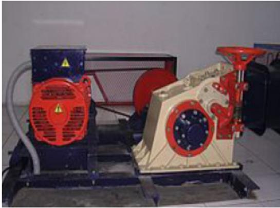
Gambar 2.1 Mikrohidro Tipe *Cross flow*
