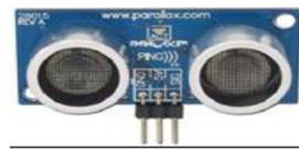
Gambar 2.3 Sensor Ultrasonik PING<sup>[20]</sup>
