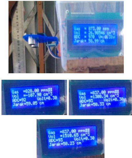
Gambar 9. Kalibrasi Sensor Ultrasonik HC-SR04
