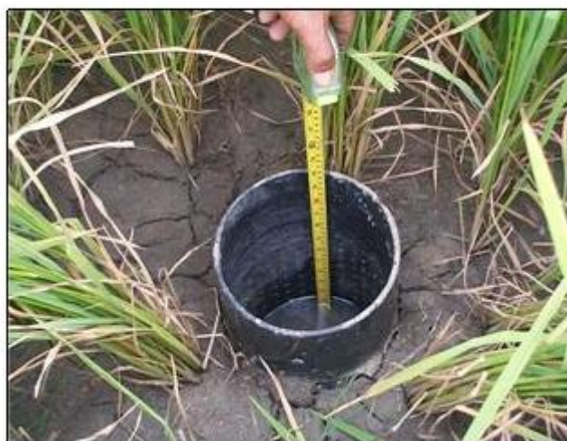
Figure 3 Field water tube to determine time to irrigate in the AWD irrigation method
