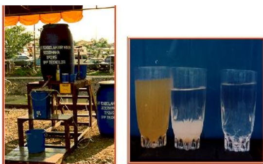
Figure 6. An example of simple water purification reactor.
