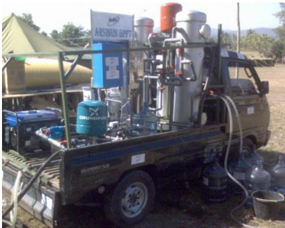
Gambar 14. Arsinum kapasitas 30 m 3 /hari (Genset 1,5 KW, Pompa, Pasir, Cartridge Filter, Ultrafiltrasi, UV Light, Ozonator).
