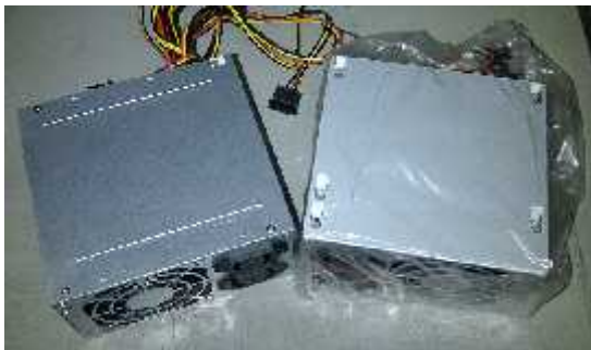
Gambar 6 : Standar Power Supply Unit.
