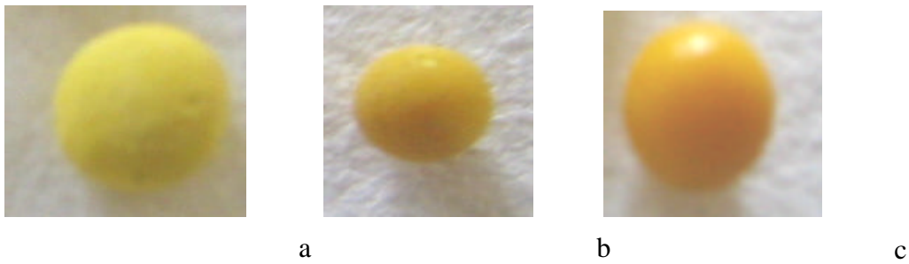
Gambar 1. Gel variasi medium (a) medium 2-etilheksanol, (b) medium CCl 4 , (c) medium minyak jarak kepyar
