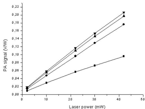
Figure 4. – Values for PA signal vs. laser power at different gas flow rates of the 100 ppm NO<sub>2</sub> concentration in N<sub>2</sub>. : 2 l/h; ? 10 l/h; ? 15 l/h; ? 20 l/h
