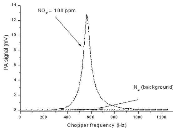
Figure 2- Resonance frequency of the PA cell
