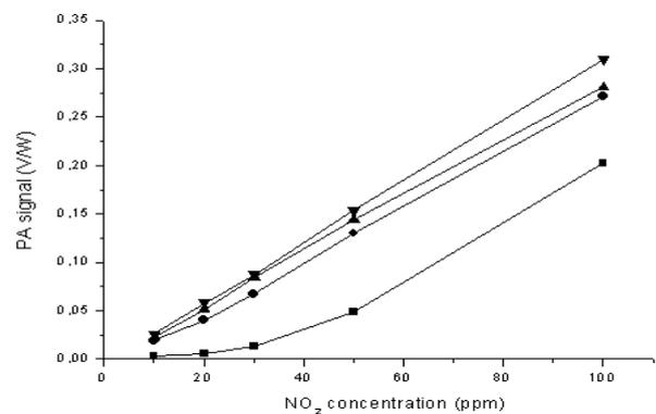
Figure 3. – Values of PA signal vs. NO<sub>2</sub> concentration in N<sub>2</sub> at different flow rates at a laser power of 42 mW. : 2 l/h; ? 10 l/h; ? 15 l/h; ? 20 l/h
