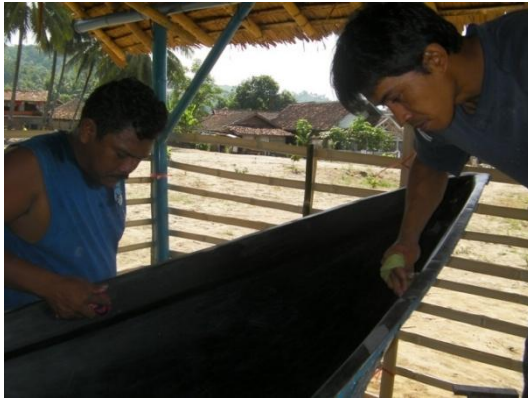
Gambar 3 Pelapisan mirror glaze/polish
