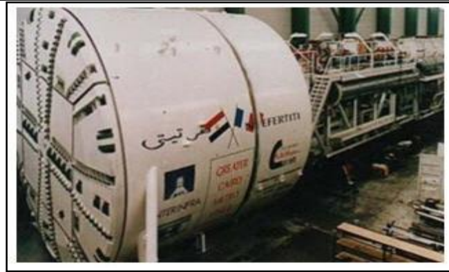
Fig. 3: The slurry TBM used in Line 3, Lot 11-c (Phase 2A), of the Greater Cairo metro (NAT 2017).
