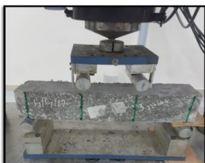
Fig. 4(a): Flexural strength test under two point loading
