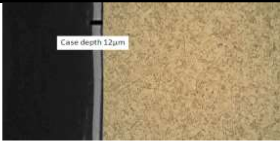
Fig.4.2: Flame hardening - 5 minutes 12 \mu m
