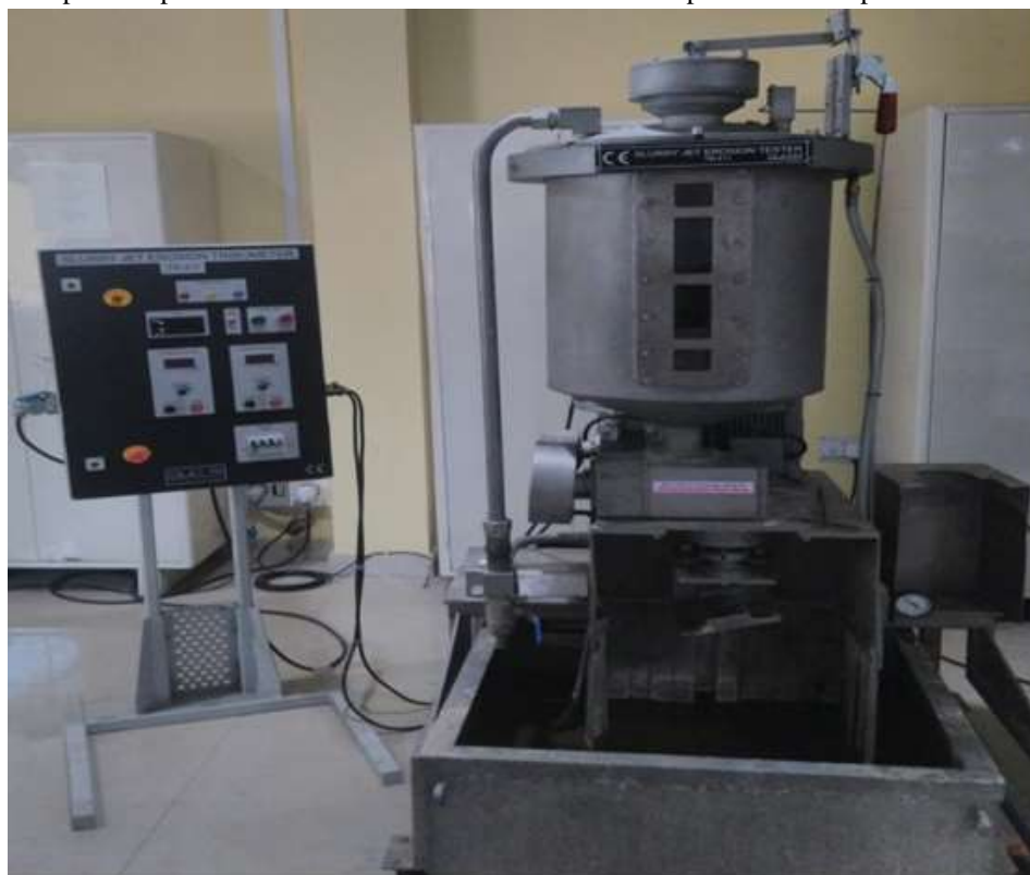
Fig.2: Test setup of Slurry Jet Erosion Tester
