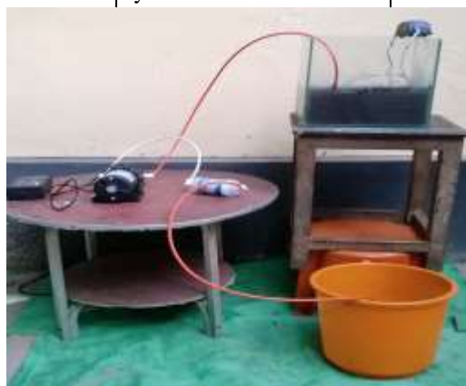
Fig.2 : Experimental setup of MBR
