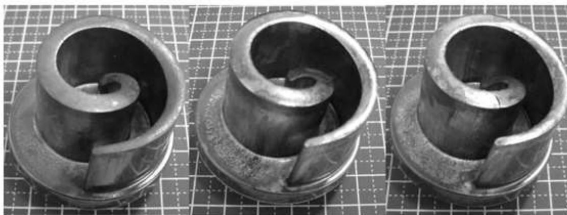
Fig.7: Forged parts (Left: AZ91, Center: AZ121, Right: AZ131)
