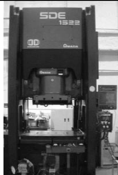
Fig.4: Servo press machine (SDE1522, AMADA MACHINE TOOLS CO.,LTD.)
