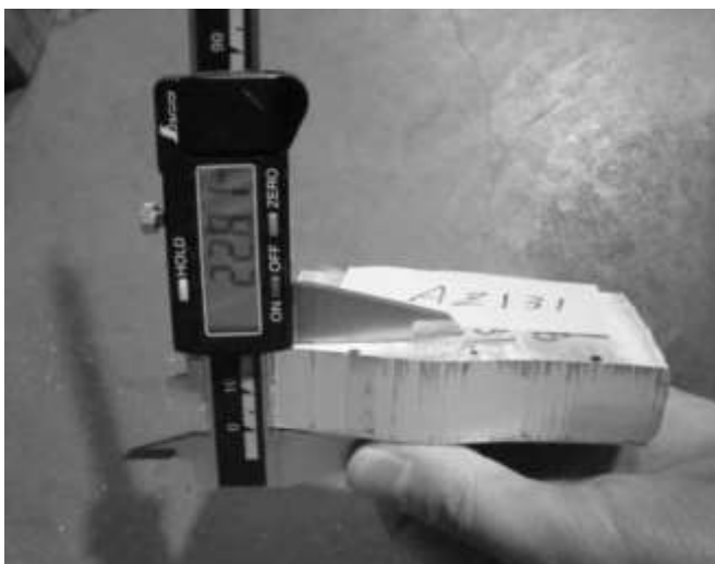
Fig.3: Cross section of roll casted AZ131 strip
