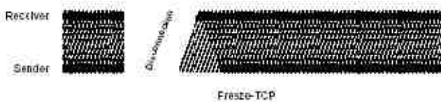
Fig.3: Increased throughput due to Freeze-TCP [13]
