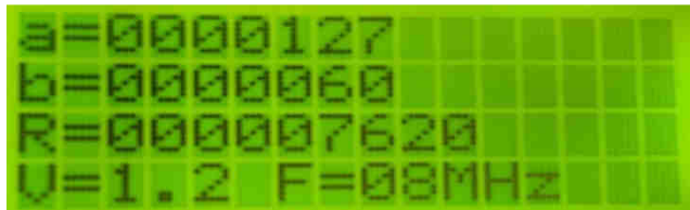
Fig.5: Multiplication result for 8-bit data by LCD.
