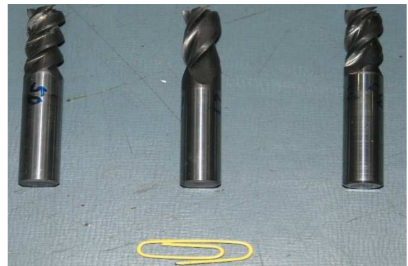
Fig.3: Endmills used in the experiment (50°, 27°, 38° Helix angles)
