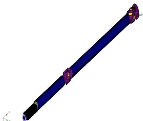
Fig.5.2: Torque of 625N.m applied at one end.
