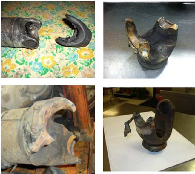
Fig.3.1: Universal coupling failure.
