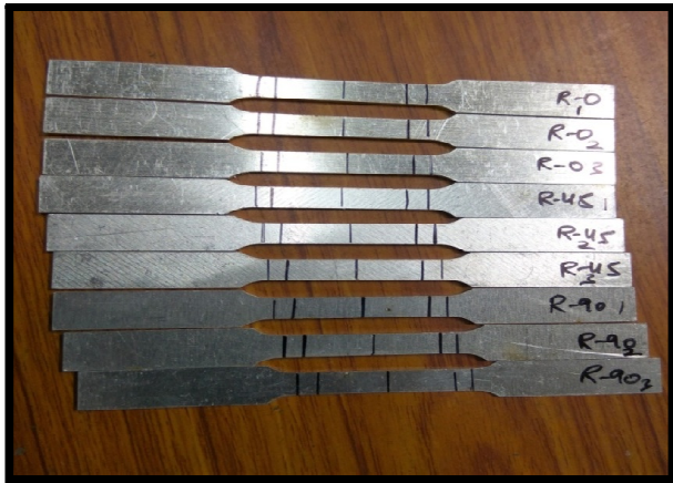
Fig.1: Specimens obtained from laser cutting machine.
