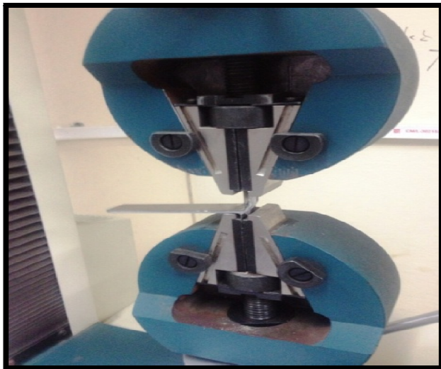
Fig.2: Instron machine used for tensile testing
