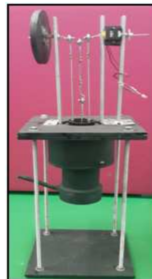
Fig 4: Flywheel with shaft attached to dynamo
