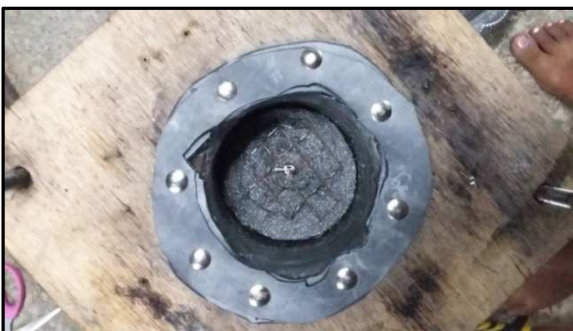
Fig 2: Setting piston inside the cylinder
