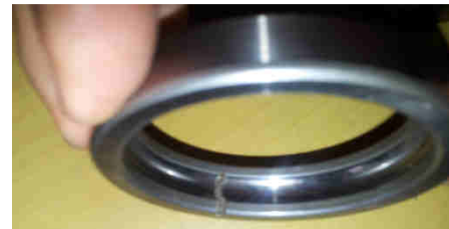
Fig.8.4: Bearing with wear of 1.5mm by width and thickness at inner race with corresponding FFT Spectrum
