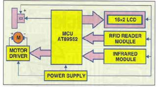
Fig 1: Block Diagram of RFID Based Parking System
