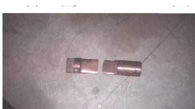
Fig.1.3: Shearing failure of key
