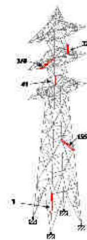
Fig. 1.6: Highlighted members whose force-diagrams are plotted
