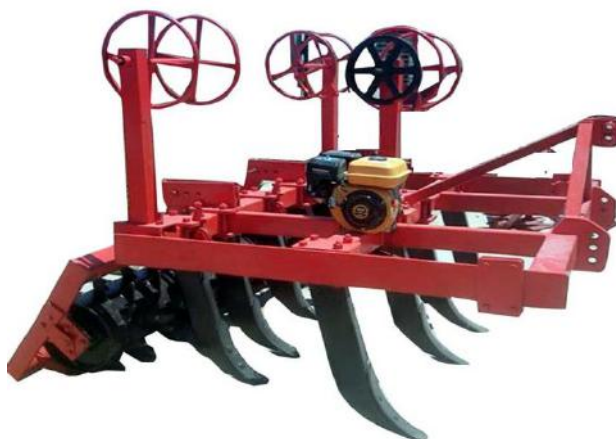
Fig.1: Combine implement used in instslation irrigation pipes
