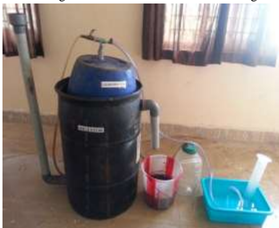
Fig.2: Lab scale model biogas digester and measurement of the biogas using water displacement method
