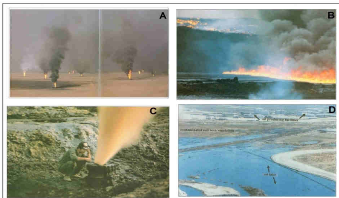
Fig.2 A & B: Oil wells are firing and dark smoke; C: A head broken well gushing oil, D: Oil lakes, Tarmat and contaminated surface at the Burgan oil field.
