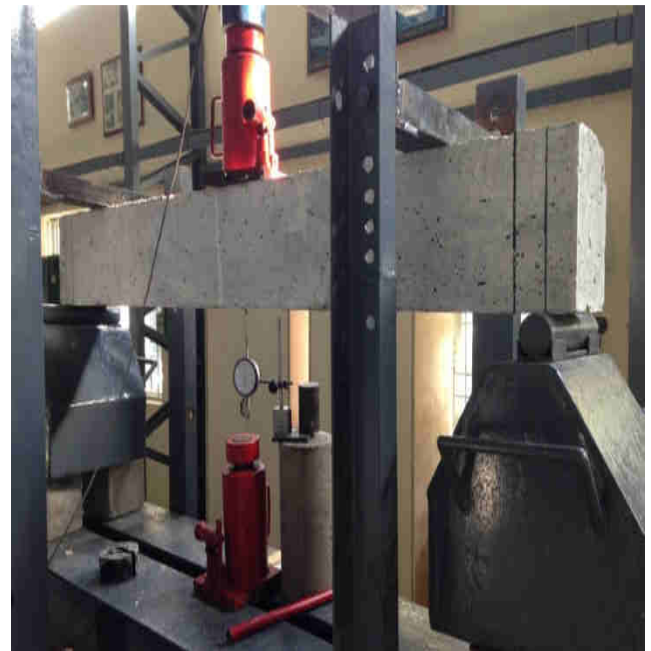
Fig.1: Test setup for Cyclic Loading
