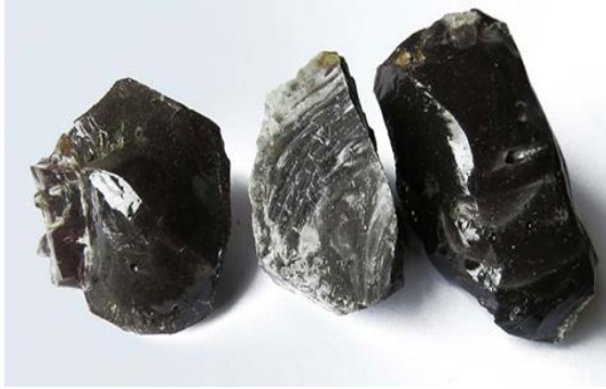
Figure 1. Slag from Blast Furnace Waste Type Glass
