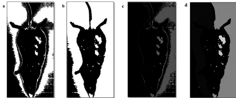
Figure 9 Segmentation method 1 on enhanced images using: (a) histogram equalization and (b) Wiener filter, segmentation method 2 on enhanced images using (c) histogram equalization and (d) Wiener filter.
