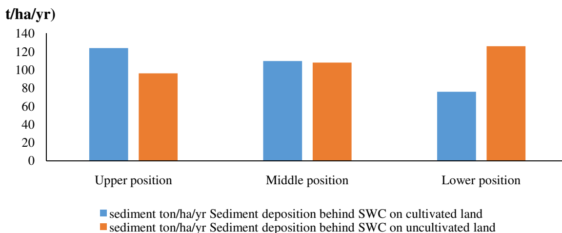
Figure 5. Sediment deposition behind SWC structures
