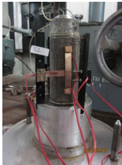
Figure 10 Soil specimen instrumented with LDTs.
