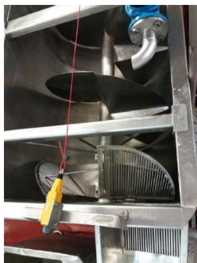
Fig. 6: Changes in the leg quarter remover from above
