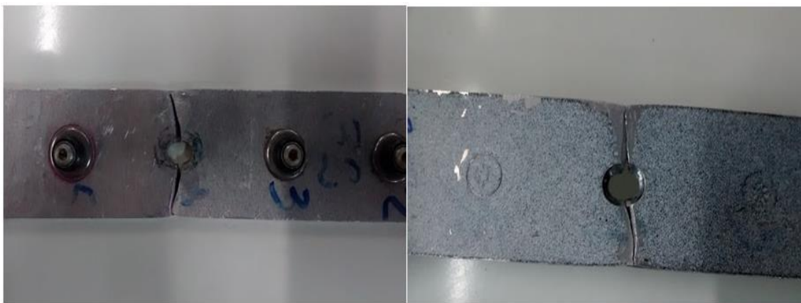
Fig.13: Top and bottom view of the failure.
